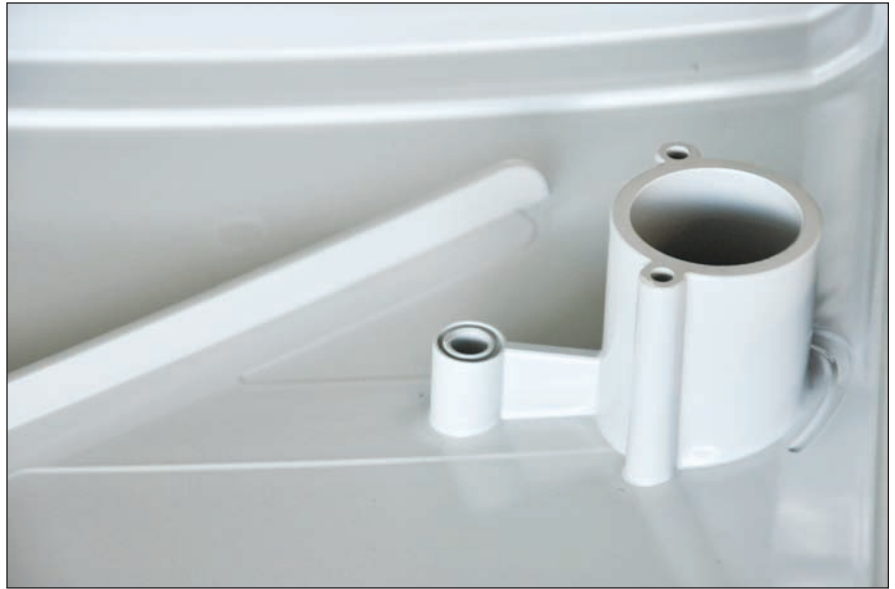
Fig. 3 – This injection-molded application illustrates the parallel use of both a flow leader and a flow restrictor. The flow leader aids resin flow to the tall corner feature, and the flow restrictor (groove) forces the resin up into the tall feature and packs it out.
